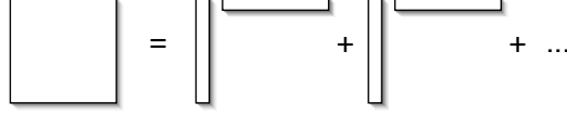
Figure 3. In HITS model, the SVD provides a 2-way decomposition that yields authority and hub scores.
