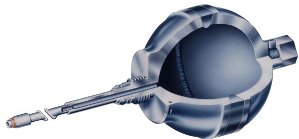
FIGURE 1. Typical Gas Reservoir
