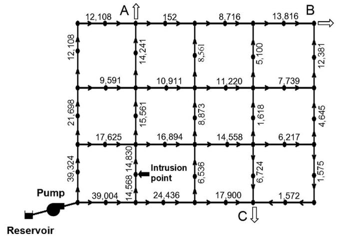
**Fig. 9.** Scenario building and corresponding EPANET setup for a  $4 \times 5$  junction simplified water distribution network for an example case. The closed and open arrows represent the intrusion and demand points (A thru C), respectively. The Reynolds number is presented next to each pipe.
