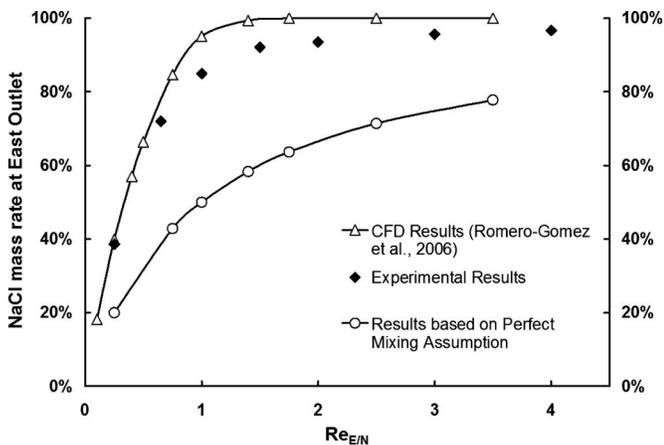
**Fig. 6.** NaCl mass rate splits from the experimental, numerical, and water quality model outcomes at different  $R_{E/N}$  (east outlet), when  $R_S = R_W$  and  $R_E \neq R_N$  (Scenario 3)
