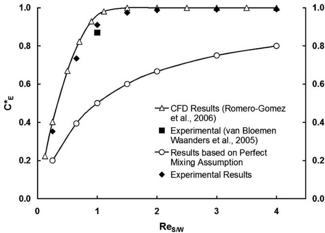
**Fig. 5.** Dimensionless concentrations from the experimental, numerical, and water quality model outcomes at different  $R_{S/W}$  (east outlet), when  $R_S \neq R_W$  and  $R_E = R_N$  (Scenario 2)
