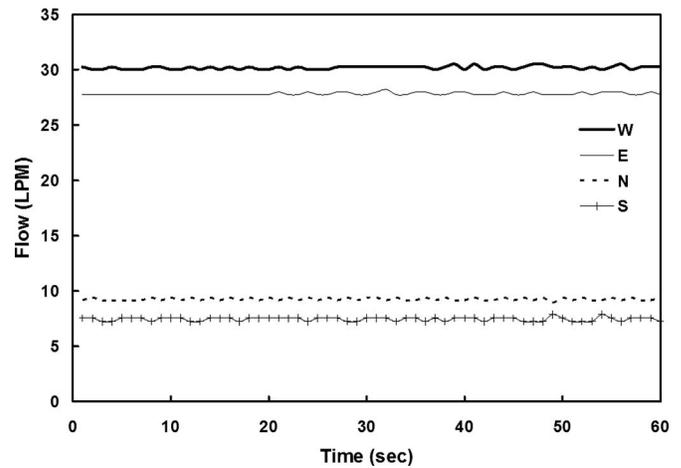
Fig. 2. An exemplary case of flow measurements:  $R_{S/W}$  and  $R_{E/N}=0.25$  and 3.0, respectively. LPM indicates liters per minute.
