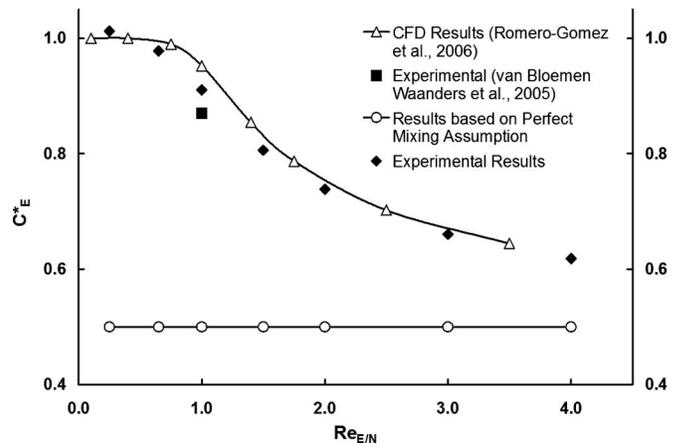
**Fig. 7.** Dimensionless concentrations from the experimental, numerical, and water quality model outcomes at different  $R_{E/N}$  (east outlet), when  $R_S = R_W$  and  $R_E \neq R_N$  (Scenario 3)
