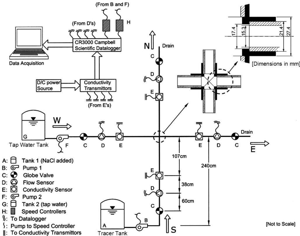
Fig. 1. A schematic of the experimental setup
