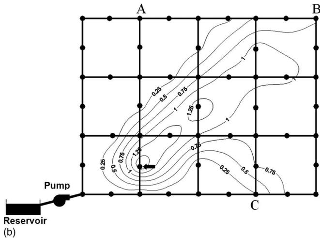
**Fig. 10.** Contours of NaCl concentration (mg/L); (a) based on perfect mixing assumption; (b) after modifications of the code. The arrow indicates the intrusion point, and concentration immediately after the dilution in the pipe is 1.77 mg/L.
