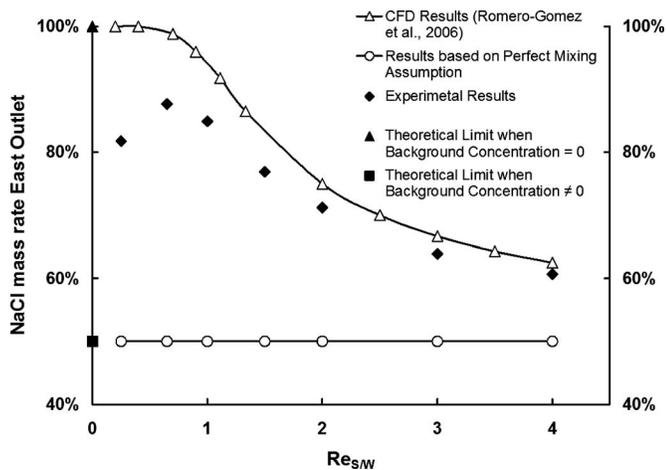
**Fig. 4.** NaCl mass rate splits from the experimental, numerical, and water quality model outcomes at different  $R_{S/W}$  (east outlet), when  $R_S \neq R_W$  and  $R_E = R_N$  (Scenario 2)
