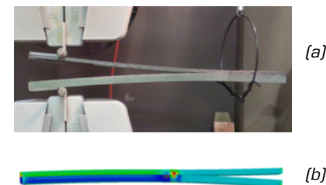
Figure 2. Example double cantilever beam (a) experiment and (b) FEA model
