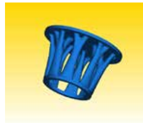
A topology optimized round table to support a uniformly distributed load. The table legs take on the shape of branching tree trunks simply by specifying material to be used optimally within the allowable space to maximize stiffness.
