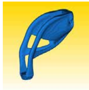
A topology optimized shape for a bracket loaded vertically and bolted to the wall horizontally.
