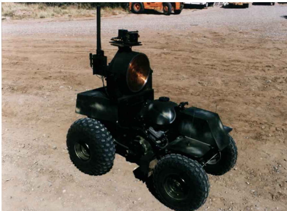
Fire Ant, an early example of a mobile autonomous armor-defeating system, uses an explosively formed projectile (EFP). Sandia continues to develop more lethal warheads for integration onto mobile platforms.
