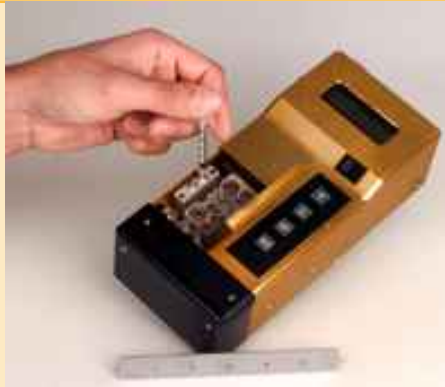
Sandia's hand-held, integrated device for analyzing liquid and gas mixtures.
