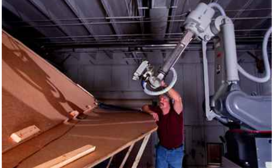
A Sandian examines a pair of cameras that provide feedback to the computer system controlling the automated paint system for the F-177 Nighthawk jet.
