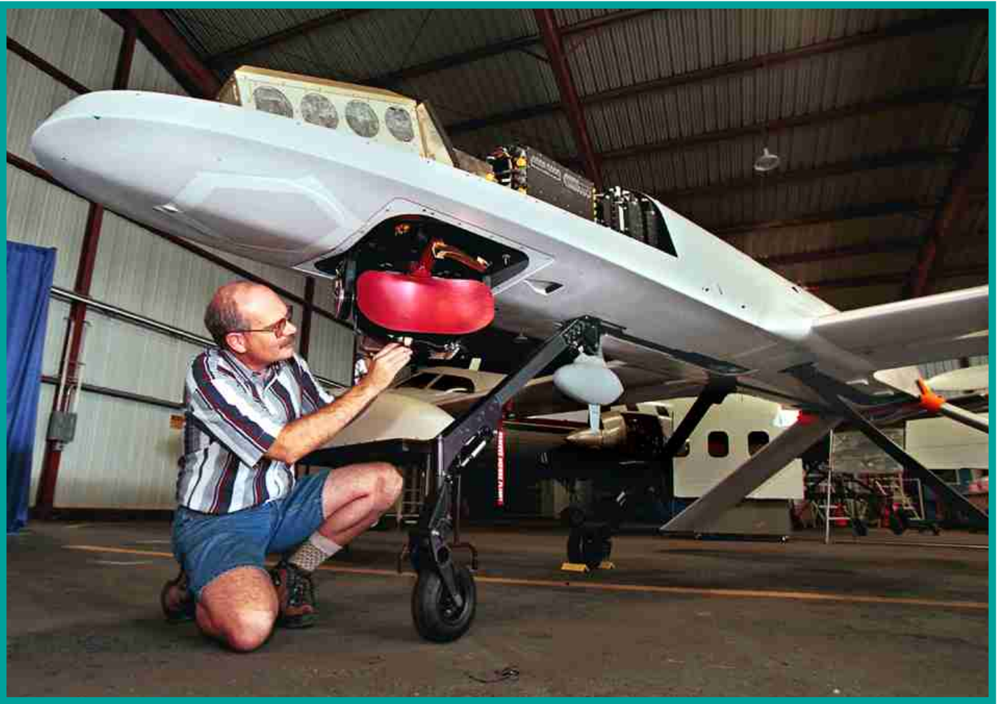
Sandia researcher Bill Hensley checks the Lynx synthetic-aperture radar (SAR) installed on a General Atomics I-GNAT unmanned aerial vehicle.
