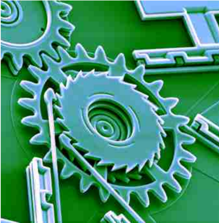
This image shows a ratcheting system fabricated in the five-level technology. Twenty of these gears fit on a period in a newspaper sentence.
