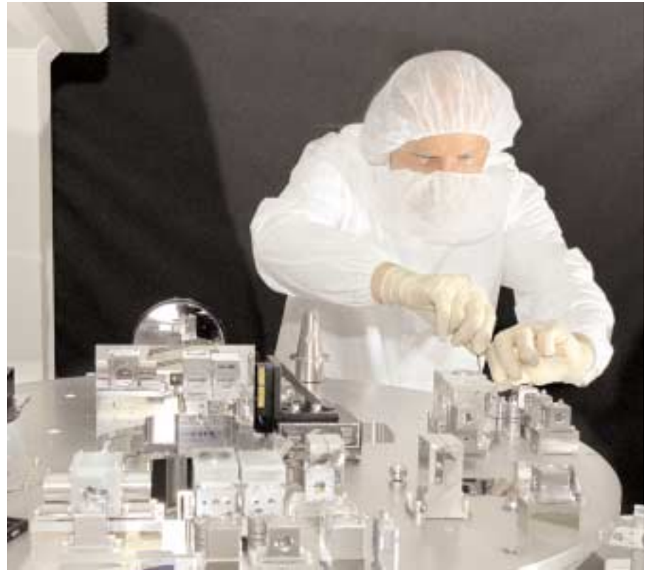
A SANDIA ENGINEER makes fine adjustments to the highly complex EUVL tool, developed by a DOE labs-industry partnership.
