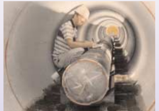
CLIFF HOWARD sits next to a line of simulated waste packages inside the 132-foot-long test assembly where the effectiveness of ventilation for heat removal is being measured for the Yucca Mountain Project.
