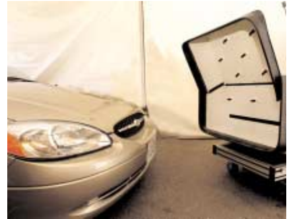
SANDIA successfully tested a prototype vehicle portal that detects trace amounts of common explosives.
