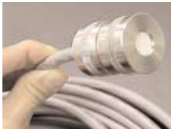
UNIQUE "sniffer" monitors volatile organic compounds in real time.
