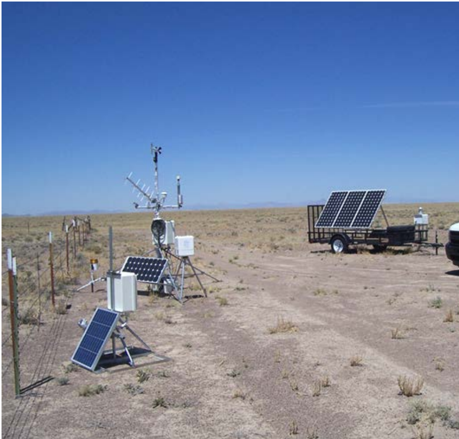
Figure 1-6. TTR solar-powered air sampler, saltation sensor, and meteorological tower (center right, foreground left, and center left, respectively) at Station 402, located along the north fence that bounds the Clean Slate 1 contamination area
