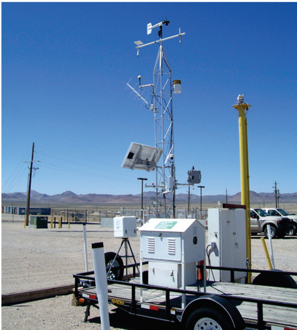
Figure 1-6. SNL/TTR Station 400 measures radiological and meteorological conditions near the ROC
