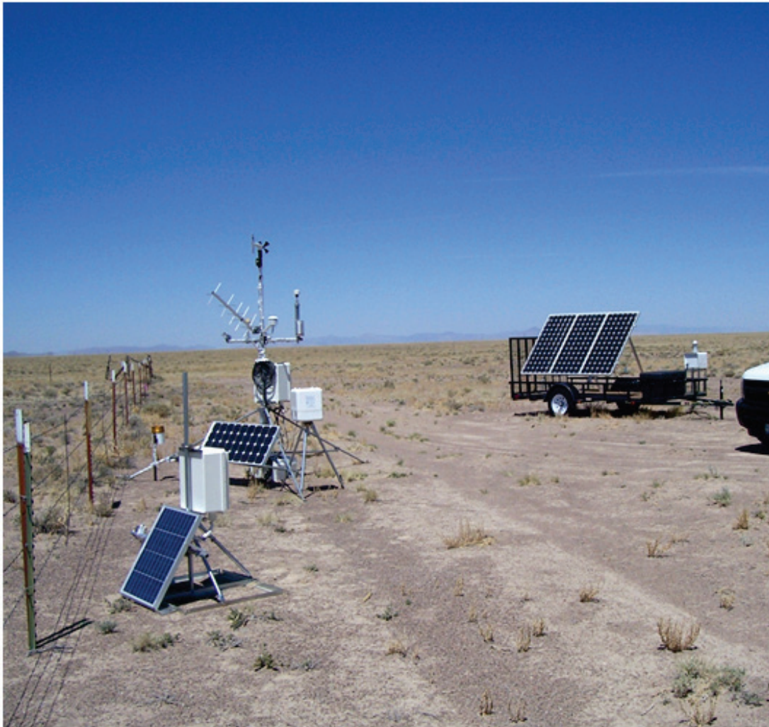
Figure 1-8. SNL/TTR solar-powered air sampler, saltation sensor, and meteorological tower (center right, foreground left, and center left, respectively) at Station 402, located along the north fence that bounds the Clean Slate 1 contamination area
