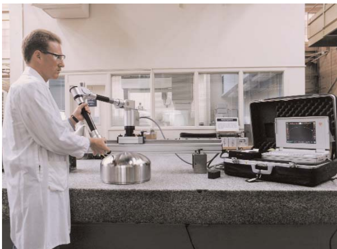
Portable CMM used to scan an ellipse on a vessel component
