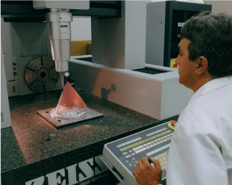
Bomb Impact Optimization System polycarbonate nose tip inspection
