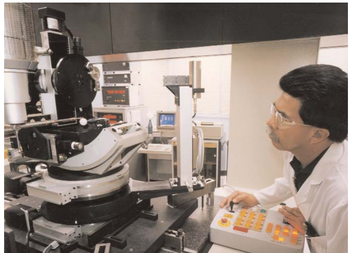
Precision alignment of a seven positioning goniometer using a CMM
