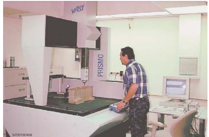
Fast scanning, variable accuracy PRISMO VAST CMM used to measure satellite hardware
