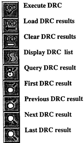
Figure 2. MEMSdrc Menu Bar
