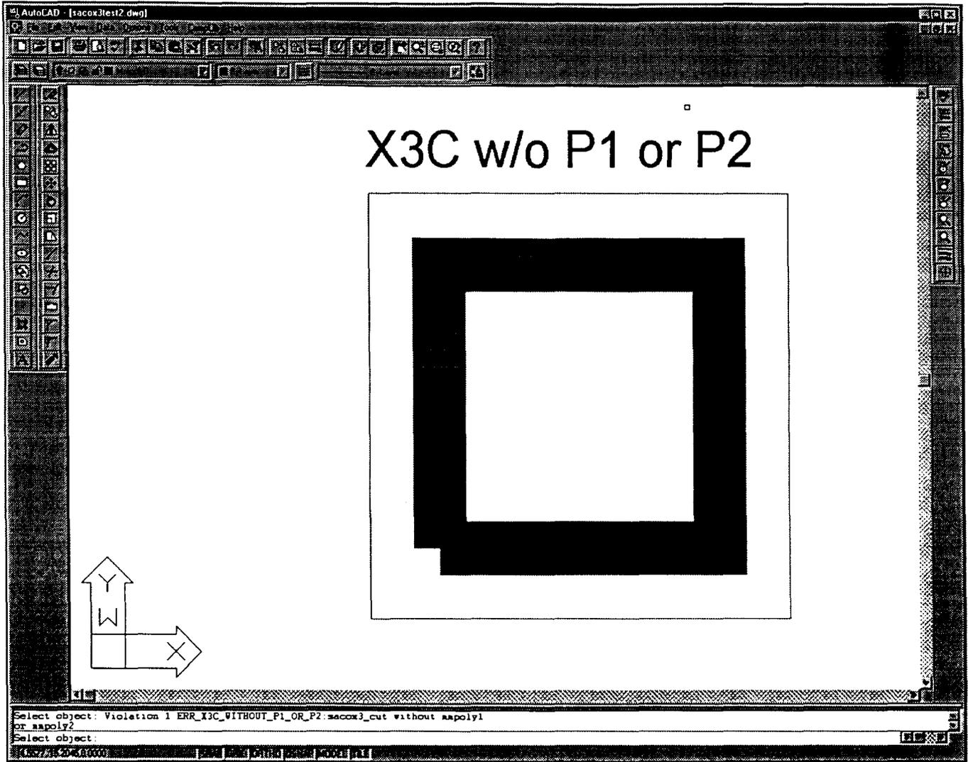
Figure 6. DRC Result Example - Missing Geometry
