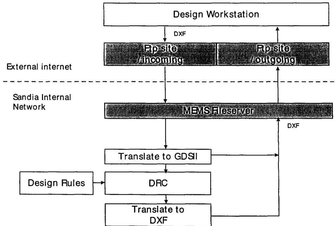
Figure 1. MEMSdrc Process Flow
