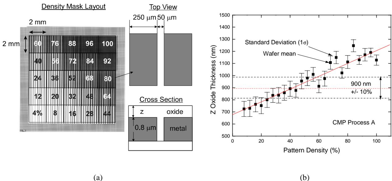
Figure 1. An example of a CMP characterization test mask used to evaluate the pattern density effect<sup>13</sup>. The mask layout is shown in Fig. 1a and the evaluation for a particular CMP process is shown in Fig. 1b.
