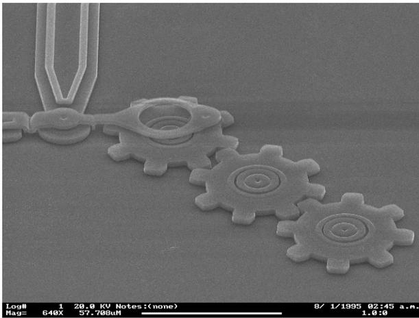
Fig. 2. SEM perspective view of the microengine output gear and two additional driven gears. Gear extreme diameter is approximately 50 micrometers and gear thickness is 2.5 micrometers.
