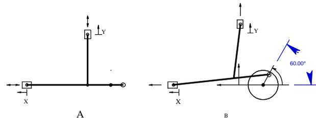
Fig. 1. Schematic illustrating the principle of operation for the microengine. Fig. 1A represents the as-fabricated or starting position, while Fig. 1B illustrates rotation through  $60^\circ$  by positive motion of both the X and Y linear actuators. The linear actuators are depicted as the rectangular boxes at the X and Y positions on the links to the circular gear.
