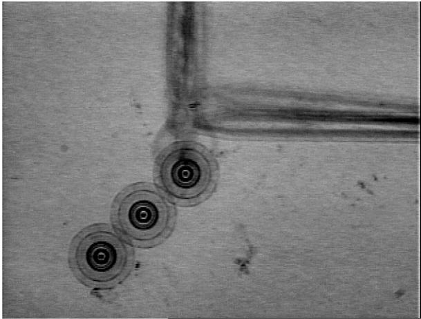
Fig. 4. Optical micrograph at 250X magnification taken during the operation of the microengine driving two additional gears at 200,000 RPM (50 micrometer gear diameter).
