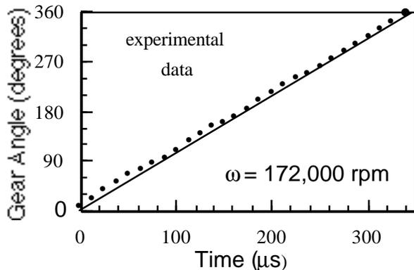
Fig. 5. Dynamical measurements of an engine output gear (driving no load) illustrates the ability to achieve controlled operation of the microengine, such as delivering constant angular speed.
