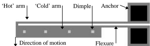
Figure 1. Schematic view of an electrothermal actuator.
