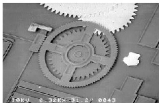
Figure 7. Rotary stepper motor. Main two-level gear adapts thermal actuator stroke to tooth pitch of standard, software-generated Sandia gears. Upper gear is planarized Poly-3.
