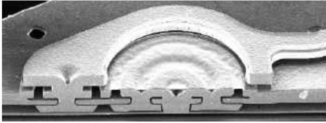
Figure 8: A scanning electron micrograph (SEM) of a linkage gear hub produced by focussed ion beam milling.
