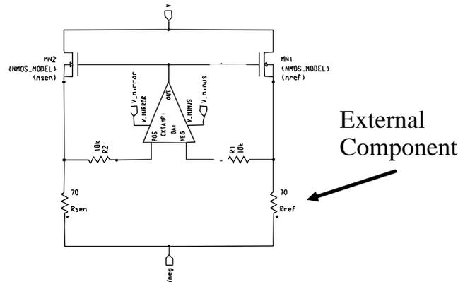
Figure 13. Schematic of the CMOS control circuit integrated with the micromachined sensing filament (labeled  $R_{sen}$ ). For the purposes of testing, the micromachined reference resistance was replaced with a 10-turn potentiometer.
