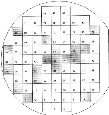
Figure 6. A wafer map from the first run showing functionality of wafer-level tests of combustible gas sensor devices. The unshaded devices are functional. The shaded devices are non-functional.
