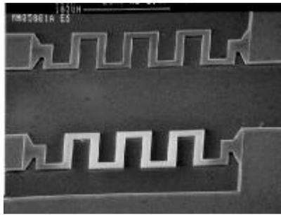
Figure 12. Plan view of two meandered microfilaments. Both filaments are fabricated of polysilicon and are 10  $\mu\text{m}$  wide and 2 $\mu\text{m}$  thick. They are elevated above the substrate by a 2 $\mu\text{m}$  air gap to provide thermal isolation of the bridge from the substrate. The lower filament is coated with a 0.1  $\mu\text{m}$  thick layer of Pt, deposited by micro-CVD techniques.
