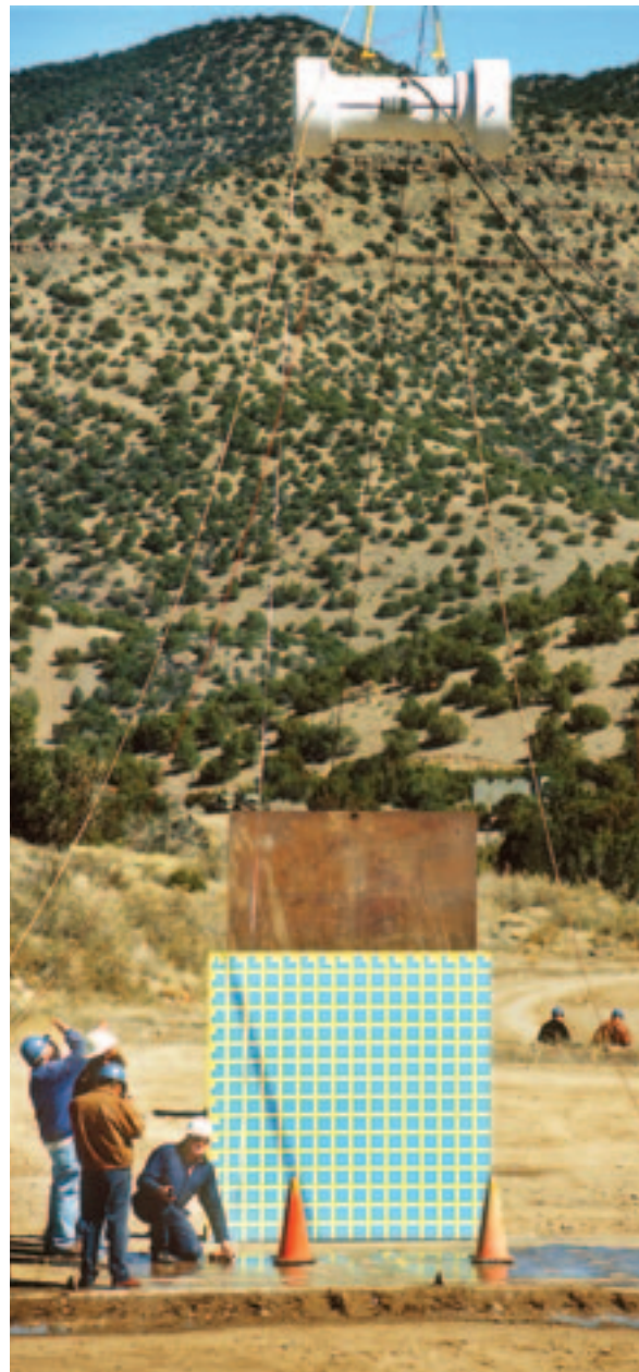
Sandia engineers prepare a commercial rad-waste transport container for a certification drop test required by the U.S. Nuclear Regulatory Commission.
