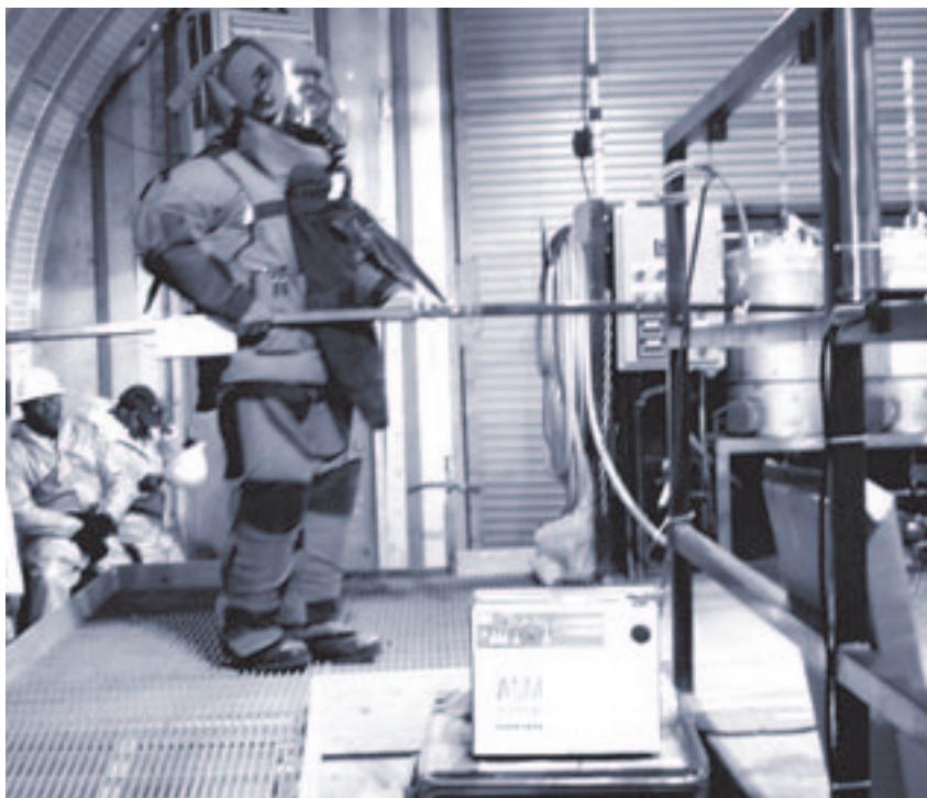
Top: A U.S. Army ordnance expert uses protective gear and a long pole to load sarin-filled bomblets into the Explosive Destruction System at Rocky Mountain Arsenal.
