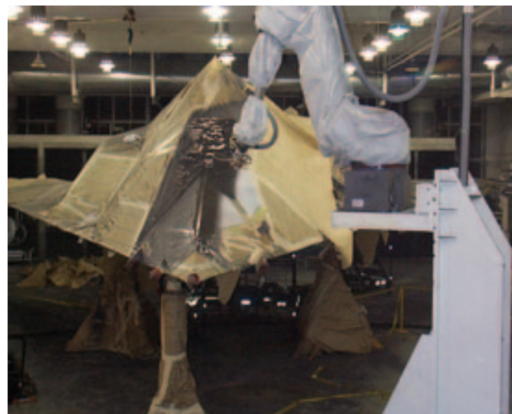
Sandia developed a robotic paint system with Lockheed Martin Aeronautics Systems for the U.S. F-117A Nighthawk.
