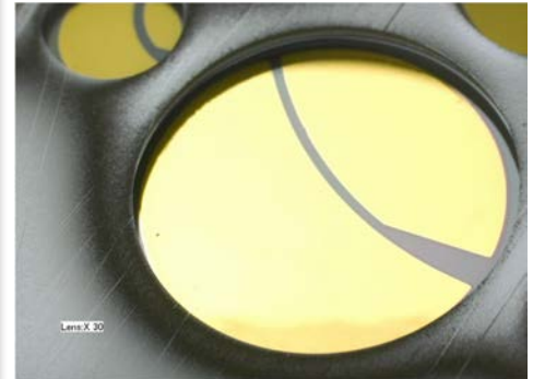
Back side of a 5 mm diameter, 5 \mu\text{m} thick PV cell after shadow mask metallization. The shape of the pads corresponds to the polarity of the PV cell.
