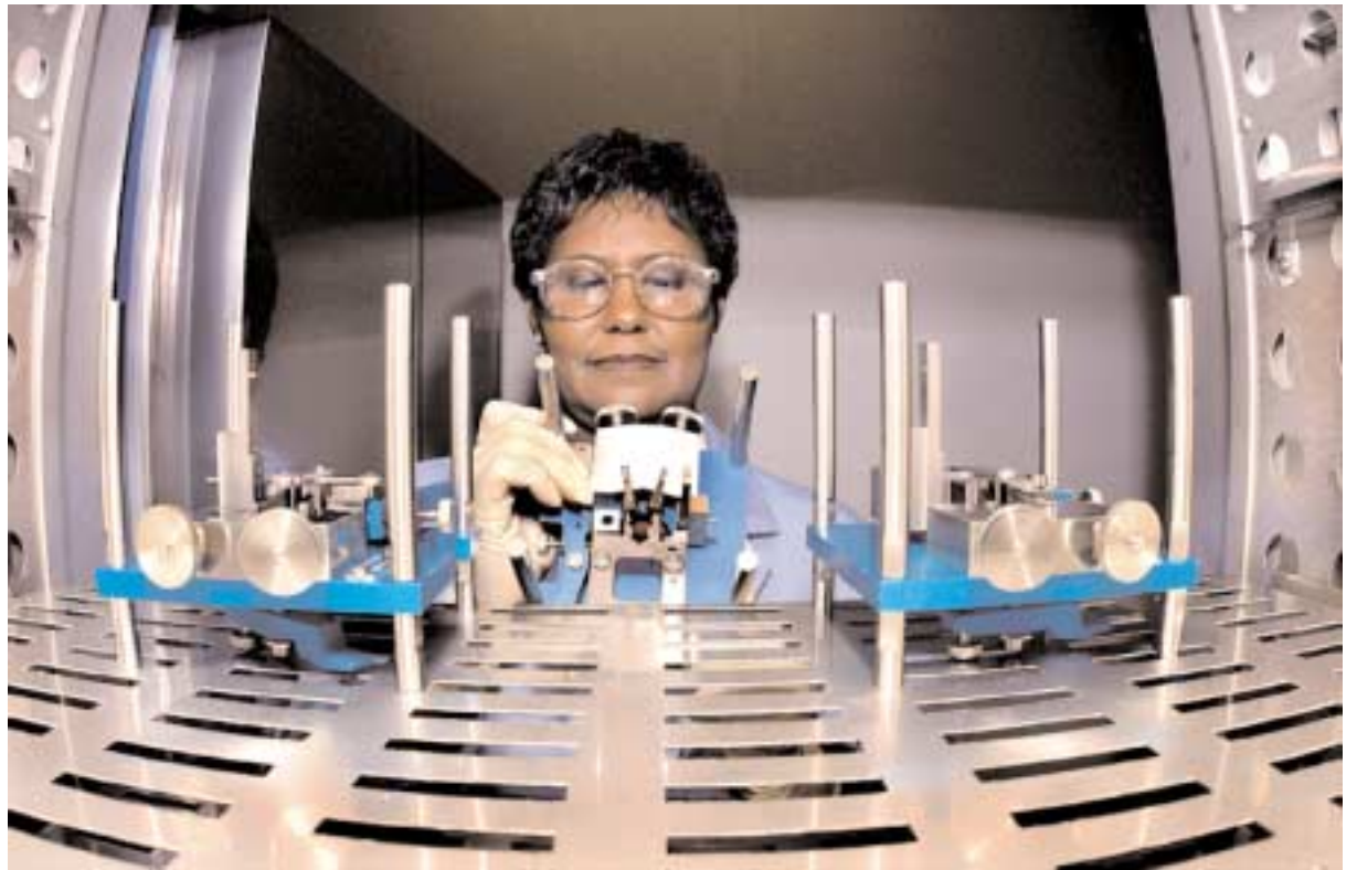
RECIPE FOR SUCCESS — Annie Nickerson (14404-4) places power supply fixtures for neutron generators into an oven at Sandia's Neutron Generator Production Facility. The latest generator was manufactured and delivered to the US Navy. (Photo by Randy Montoya)
