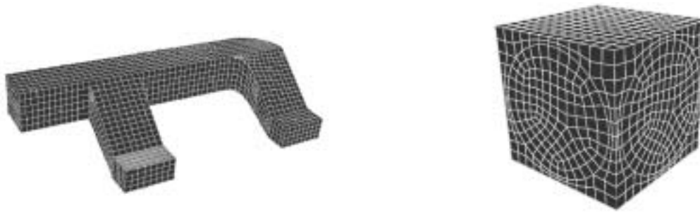
Figure 4. Examples of all-hex meshes generated automatically by the Geode algorithm.
