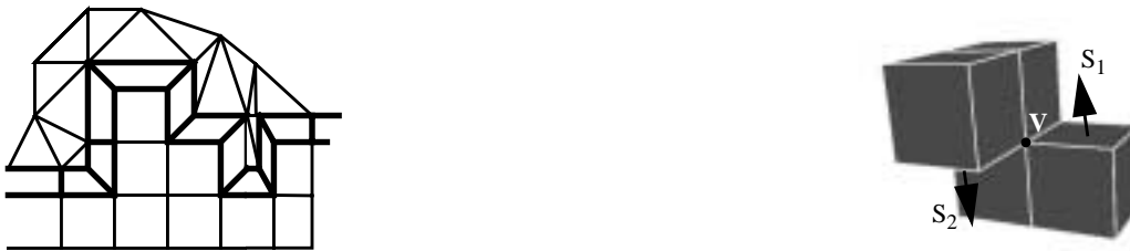
Figure 9. Interface angles affect the quality of the geode-templates. Right, in three-dimensions it may be impossible to create a buffer layer: Suppose interface node V has six attached interface faces as in the figure. Since no point can see both of S_1 and S_2 , one of the geode-templates attached to S_1 or to S_2 must have a non-positive jacobian at V .
