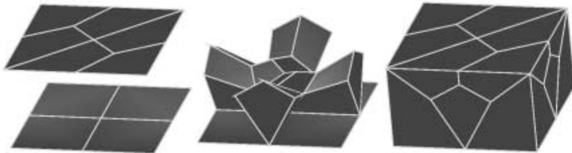
Figure 1. The all-hex geode-template: Left, the diced tet and hex interface; middle, the heart of the geode; right, the boundary of the template.
