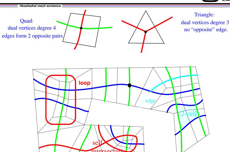
A quadrilateral mesh and the corresponding STC.
