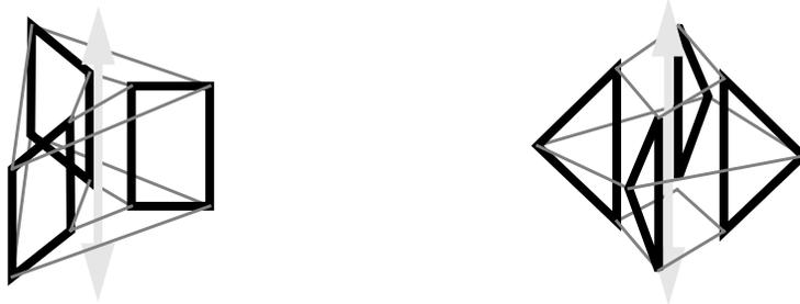
Figure 4. Two quadrilateral meshes of the surface of a torus. The axis of symmetry is vertical. Left, cycles in the non-trivial homotopy class have even parity and a hexahedral mesh of three elements is obvious. Right, cycles in the non-trivial homotopy class have odd parity, and no hexahedral mesh exists. Note that both surface meshes otherwise have the same combinatorial structure: the only difference is what is considered the inside and outside of the torus.
