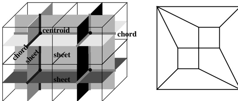
Figure 2. Right, the spatial twist continuum (STC) for a mesh of four hexahedra. Left, a quadrilateral surface mesh of a convex, planar-faceted polyhedron that satisfies conditions **a-f** above but has an odd (9) number of quadrilaterals. Hence no hexahedral mesh respects it. The ninth face forms the base of the figure and is bounded by the large outer square.
