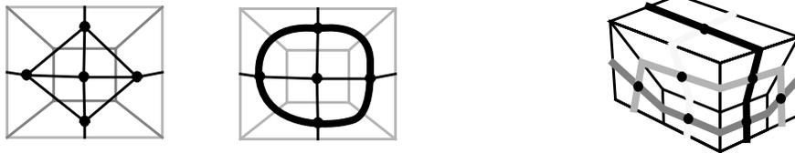
Figure 1. Left, the dual of a portion of a quadrilateral mesh. Center, a chord of the STC drawn with a wide line width. Left shows a perspective view of the loops of a closed-surface mesh.
