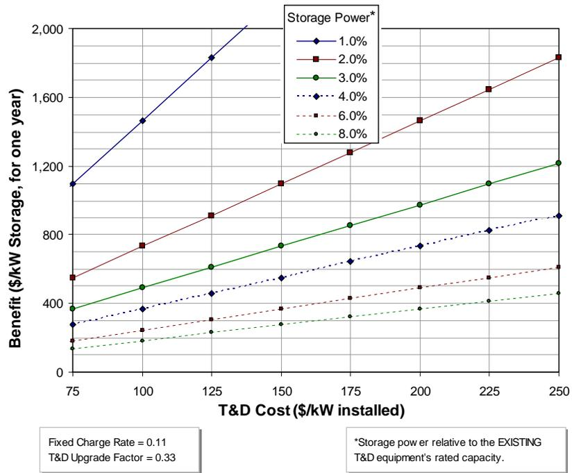
Per the figure, if DER capacity equal to 4% of the T&D equipment’s load carrying capacity (labeled as *storage power* in the figure) can be used to defer a relatively expensive T&D upgrade with an installed cost of \$125/kW (as shown on the X-axis), then the single-year deferral benefit is about \$480/kW of DER capacity. That is the benefit for *one year* of deferral. If deferrals or life extensions are multi-year, then the benefits for each year are additive.
