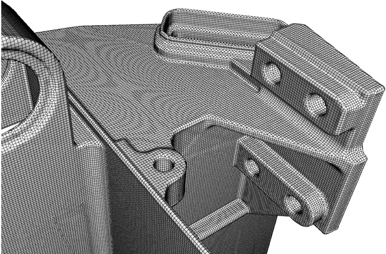
Figure 2. Hex mesh generated using the Sculpt overlay grid procedure
