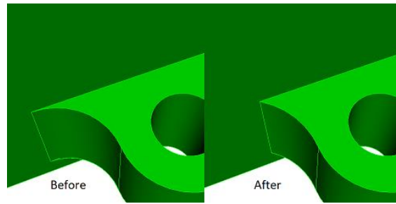
Figure 4. Blunt Tangency Tweak -- Material Removed
