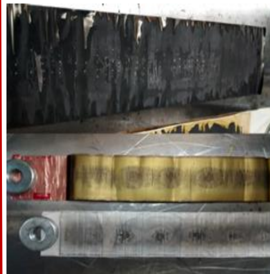
Electrodes after Cycling + Overcharge
