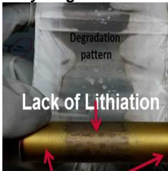
Electrodes after Cycling
