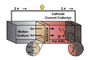
chemistry solutions at critical charge transfer interfaces and in the molten salt catholyte to enable a 10X improvement in current density, a 25X increase in usable battery capacity, and a >10X increase in battery lifetime at 110°C. Targeting publication of these dramatic improvements in Nature Energy, these advances represent important progress toward Na-based safe, low-cost, long-lifetime grid-scale storage.
