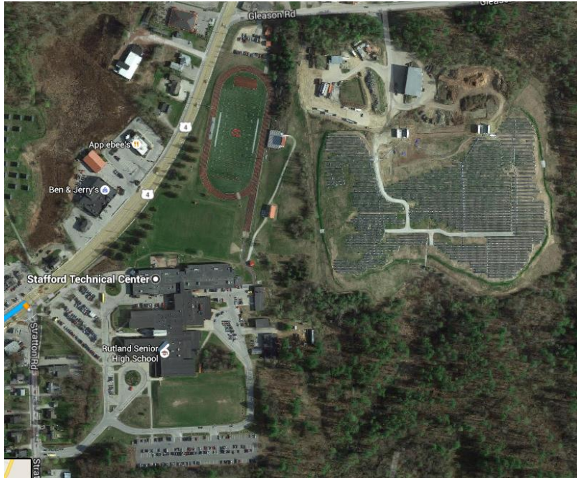
Figure 11. Photo showing Stafford Hill microgrid, adjacent high school and Stafford Technical Center. Batteries are in the four containers at the top of the solar field. There are two containers to the left and two containers to the right.
