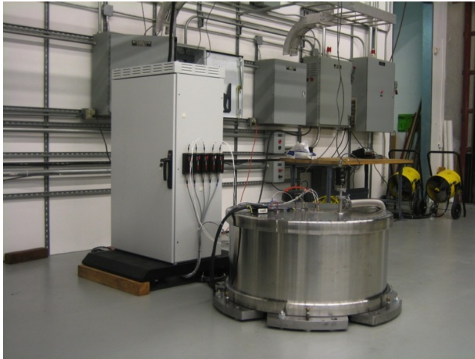
Figure 14: Amber Kinetics, first generation flywheel system [11].
