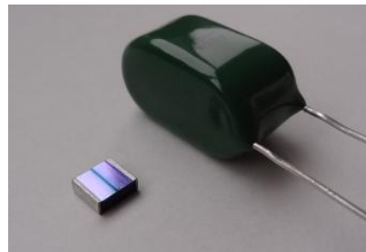
PML Chip compared to MKT type film capacitor (35v 10 \mu F)*
