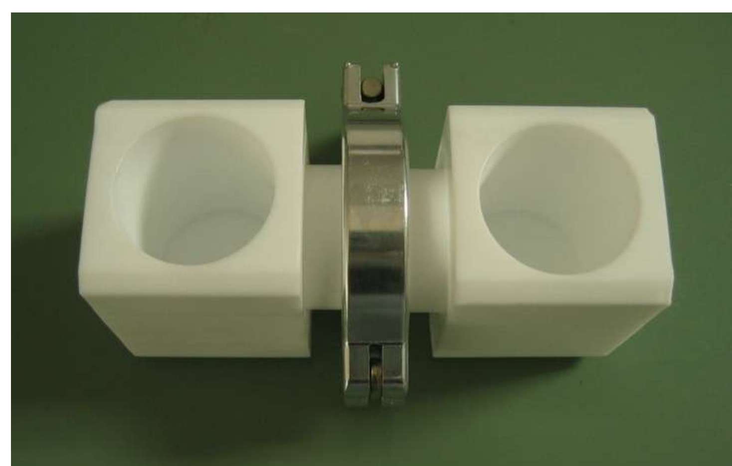
Two-compartment cell used for vanadium ion permeation tests
