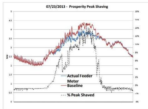
Figure 7 PNM Prosperity ESS peak shaving after optimization
