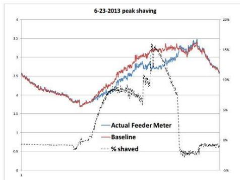
Figure 6 PNM Prosperity ESS prior to peak shaving optimization
