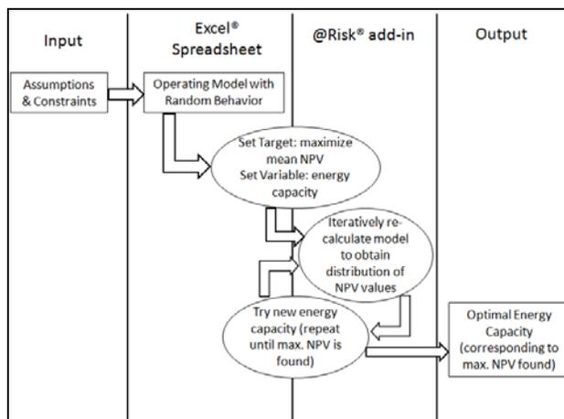
**Fig. 2.** Graphic representation of the simulation and optimization process used to find the optimal energy-to-power ratio of a flow battery performing an area regulation application.
