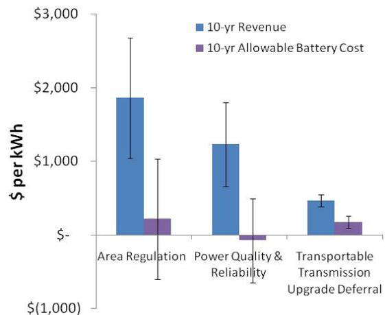
Fig. 2. Revenue and allowable battery cost for three down-selected grid energy storage applications.
