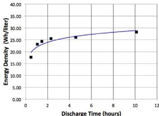
**Fig. 2. Energy density of the Aquion Energy electrode stack as a function of discharge time.**
