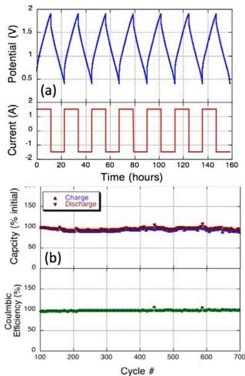
**Fig. 3. (a) Battery current and voltage profiles as a function of time for deep-discharge constant-current cycle life testing. (b) Cycle life results for 15 months of deep-discharge testing for a representative test fixture. These data indicate the long-term stability of the battery chemistry.**
