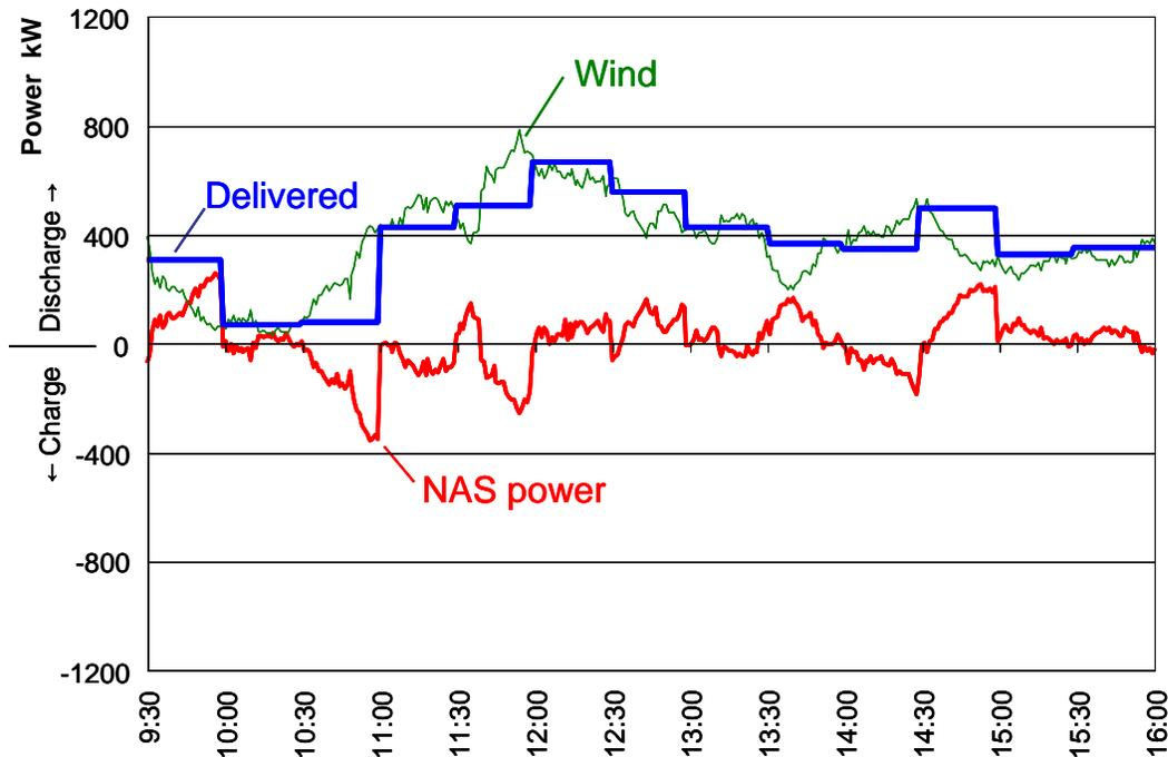
Figure 2: Wind Leveling, 1 MW Wind & 1 MW NAS battery.
