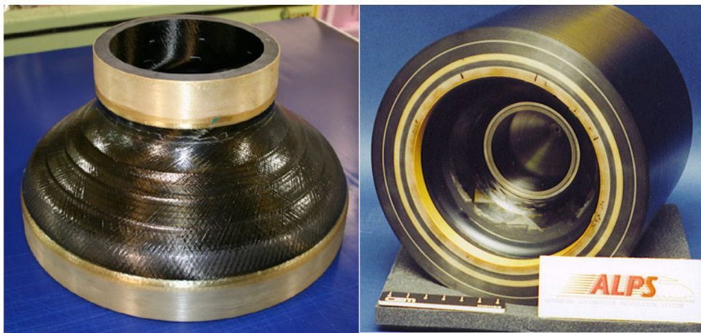
Figure 3. Composite arbor and subscale dual arbor test rotor
