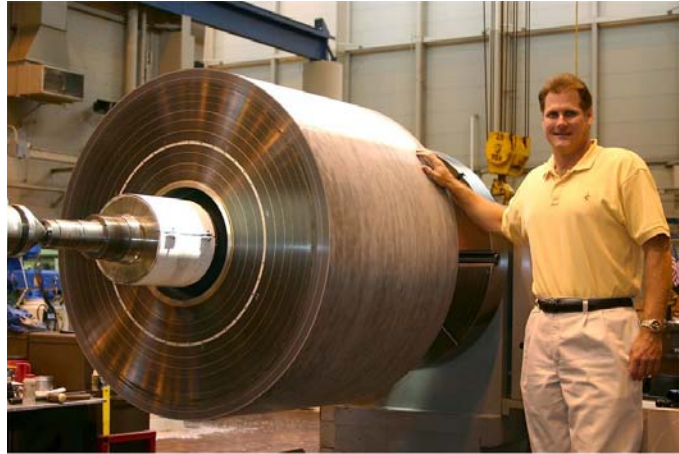
Figure 2. 480 MJ composite flywheel rotor during construction
