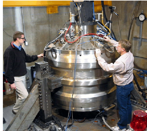
Figure 8. ALPS flywheel in spin testing bunker facility
