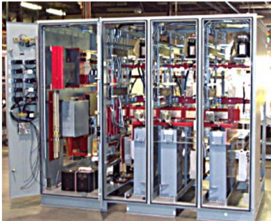
Figure 5. ALPS FESS power converter in fabrication
