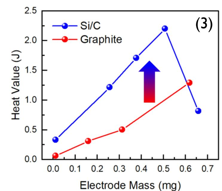
Increased energy density could be detrimental to safety in event of failure
