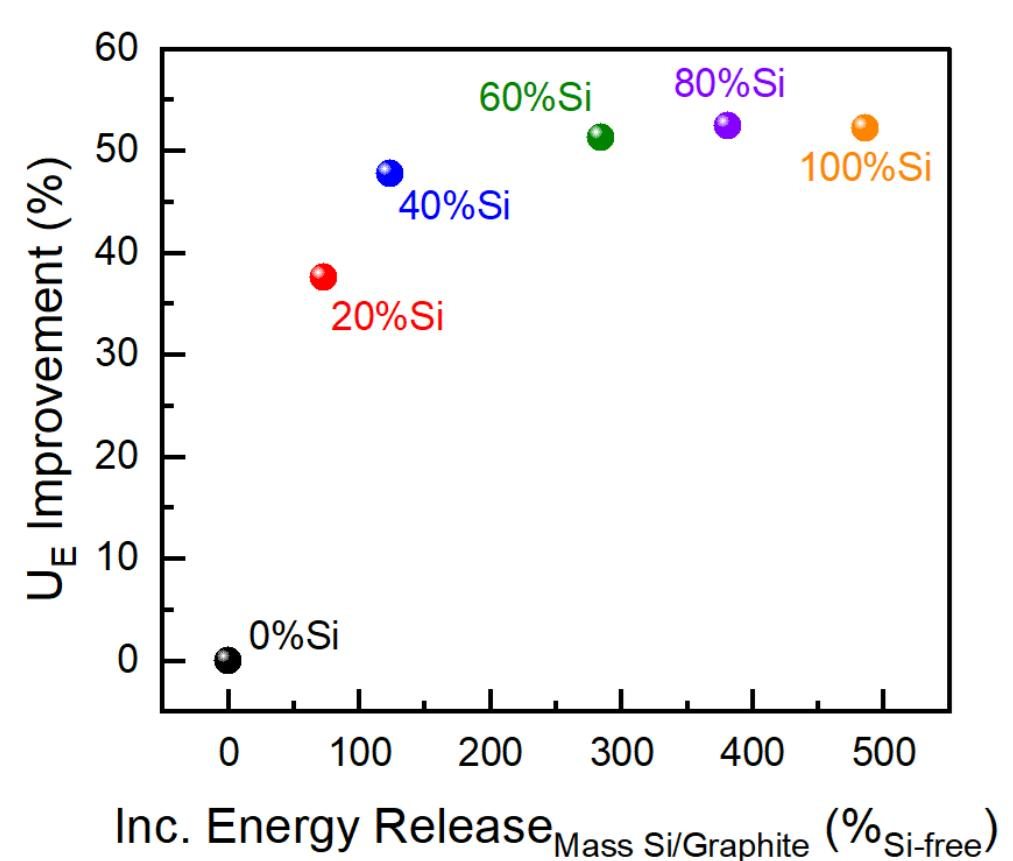
By energy released (relative to graphite) against the % improvement in energy density (U<sub>E</sub>), we can determine that **20-40% Si** provides best balance of safety and performance
