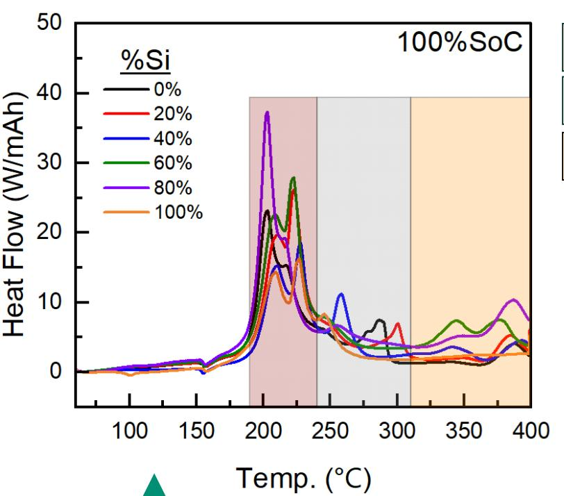
Energy release differs significantly based on normalization
