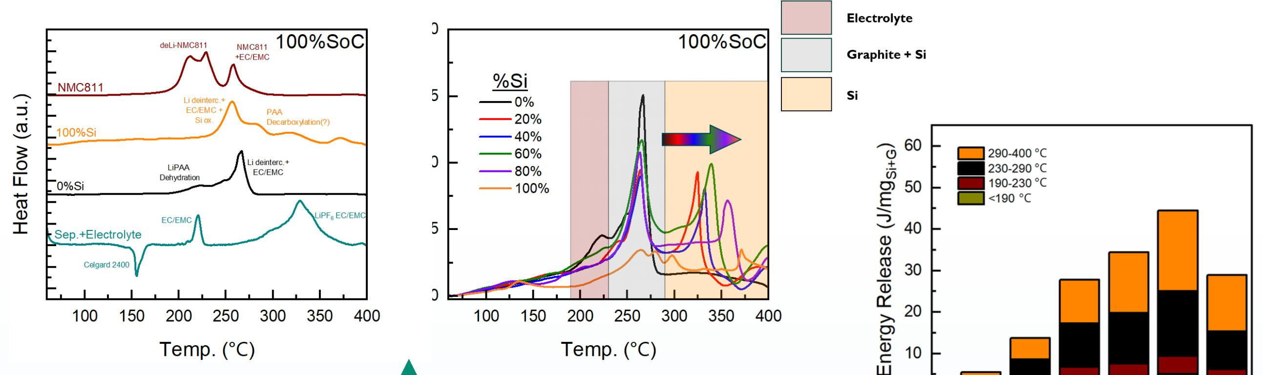
Li-C and Li-Si show similar response at ~260°C, but an additional peak >300°C is visible in the composites
