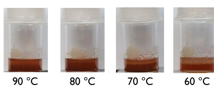
We screened >12 inorganic molten salt systems to determine melting point and phase stability. Adding select Lewis bases at 10-20 mol% enables our AlCl<sub>3</sub>-NaI based salt to remain molten at 60 °C.
