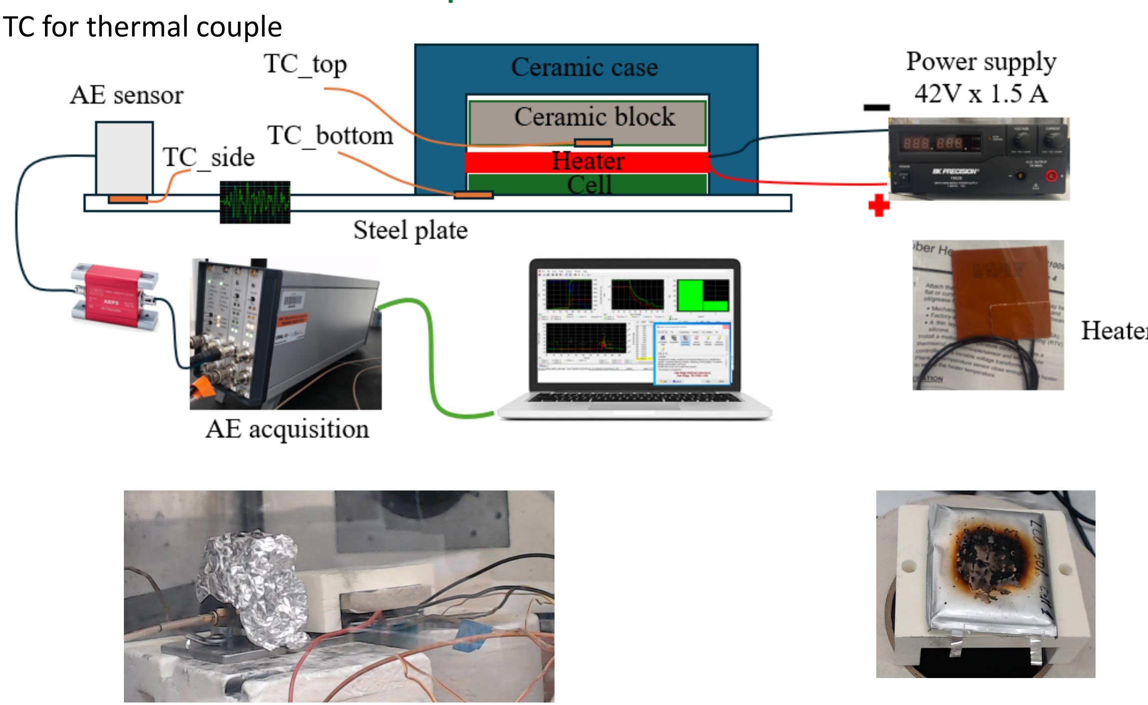
Test configuration in a venting chamber
