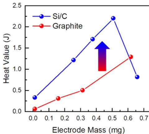
*Mixing Si with graphite results in greater heat release than graphite alone*
