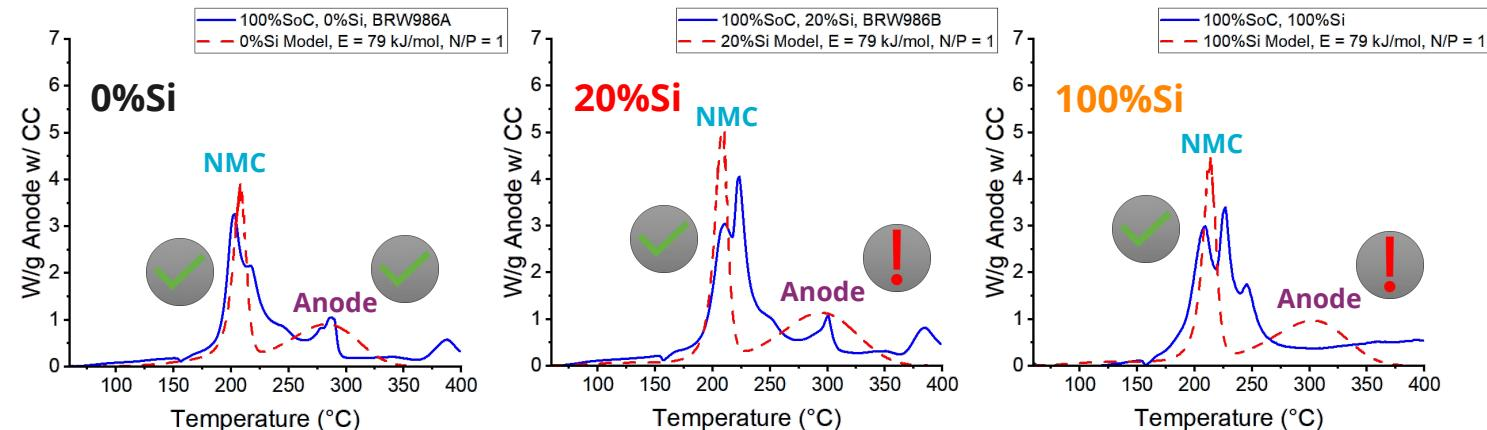
***Mixture of Si and Graphite results in unexpected deviations from modeled behavior in anode that can be explored by changing the model***
