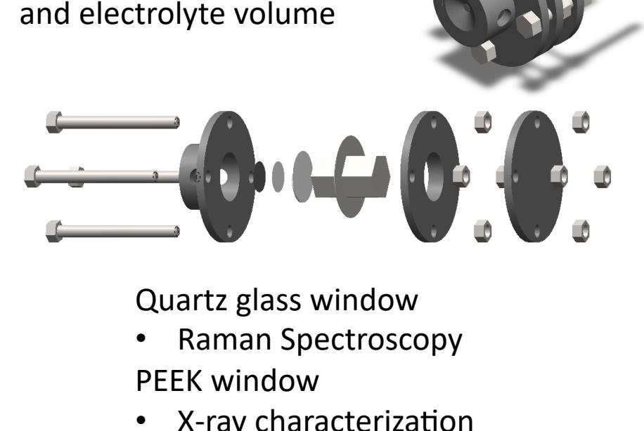
We have begun a corresponding study of the effect of compression (e) and electrolyte volume (f) on Zn-CuO cells developed at SNL. In parallel we are augmenting our previous findings on the CuO cycling mechanism with *operando* Raman spectroscopy experiments.<sup>3</sup> These have required development of a windowed battery cell with controlled compression for spectroscopic characterization of alkaline systems (g).
