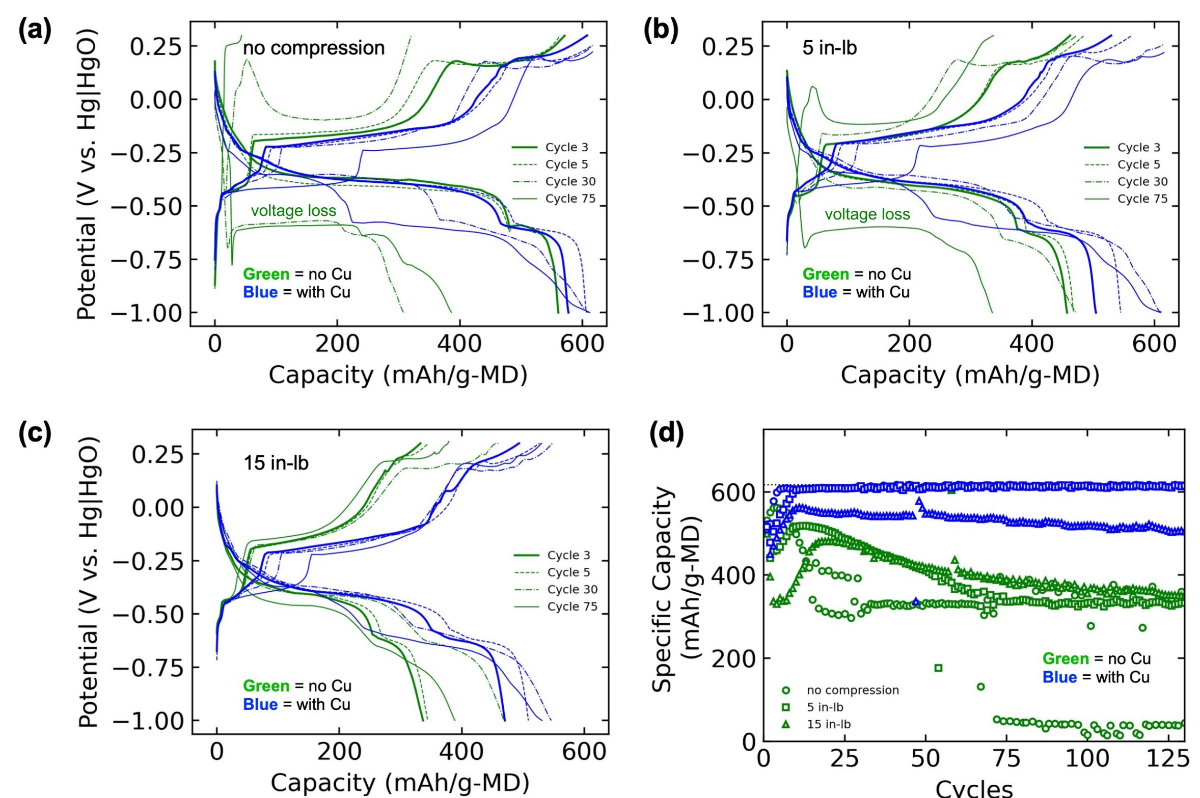
Compression is an important variable often overlooked in research on rechargeable alkaline batteries. We accomplished an analysis of the effect of compression on the alkaline MnO<sub>2</sub> cathode. Two sets of additives were considered: **MnO<sub>2</sub>+Bi<sub>2</sub>O<sub>3</sub>** and **MnO<sub>2</sub>+Bi<sub>2</sub>O<sub>3</sub>+Cu**. Including Cu has been shown to extend cycle life in the past.<sup>2</sup>
