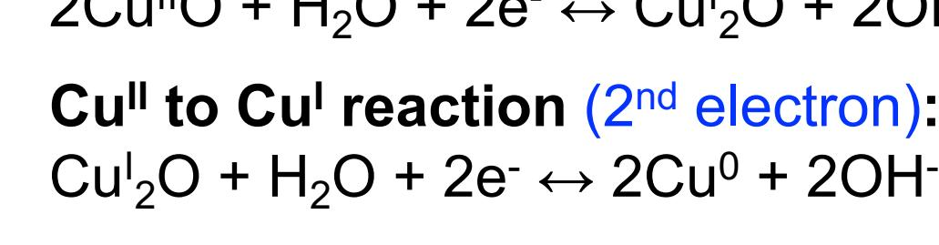
Being able to reversibly cycle 2 electrons imparts high specific capacity to these materials: MnO<sub>2</sub> being **617 mAh/g** and CuO being **674 mAh/g**. These large capacities rely on dissolution of intermediate materials and is enabled by the alkaline electrolyte. This work seeks to maintain these capacities over many cycles, to develop successful batteries for the grid.
