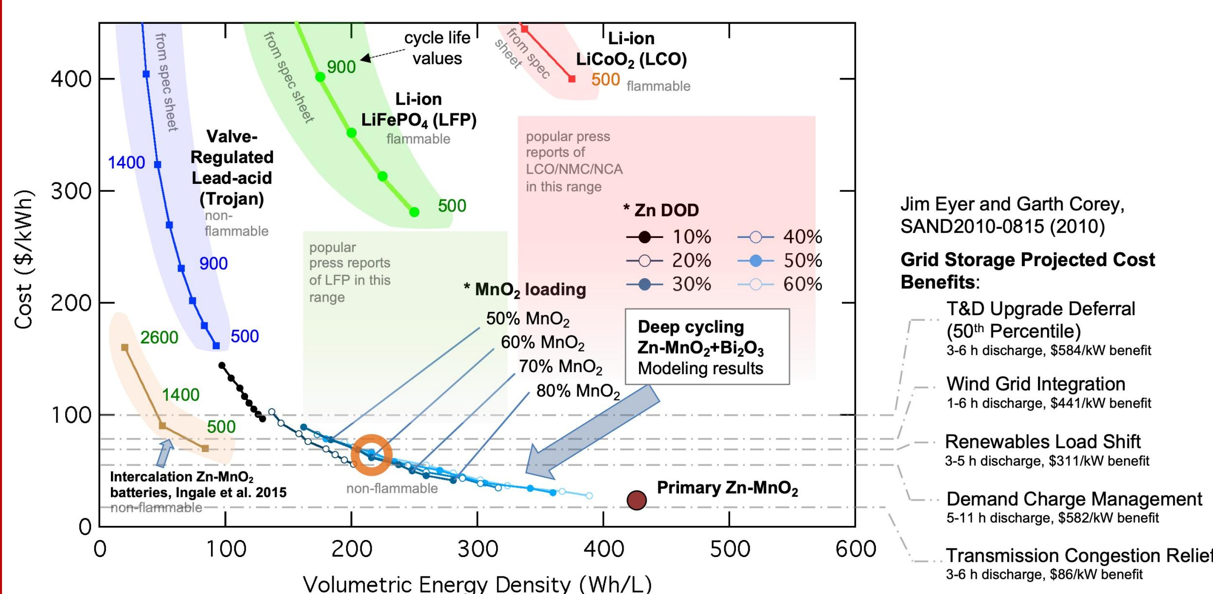
Alkaline electrolyte systems enable cathodes that can reversibly cycle 2 electrons in depth. The plot above shows analysis of the alkaline Zn-MnO<sub>2</sub> system using materials cost (\$/kWh) on the y-axis and energy density (Wh/L) on the x-axis.<sup>1</sup> In general, energy density will be highly limited by the cathode capacity. The red circle shows a design target for grid batteries with cost <60 \$/kWh and energy density >200 Wh/L.
