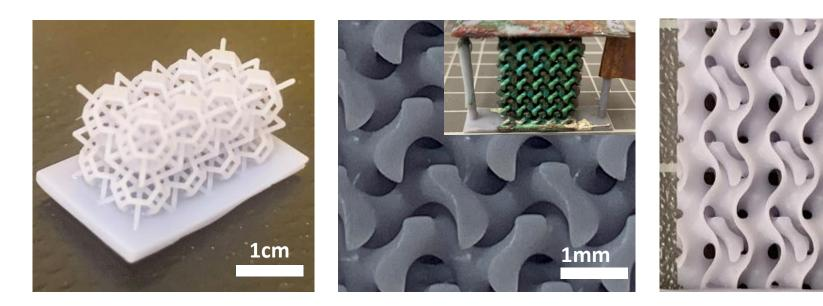
**Selective electrodeposition** of Zn onto Kelvin cells
