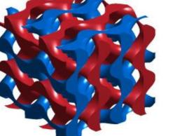
**Gyroid sheet-strut** interpenetrating
