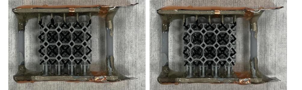
Selective electrodeposition of MnO<sub>2</sub> onto BCC cells
