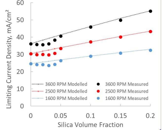
$$i_l = 0.62 nFC \omega^{1/2} v^{-1/6} (D + r^2 \Phi \omega^m)^{2/3}$$
