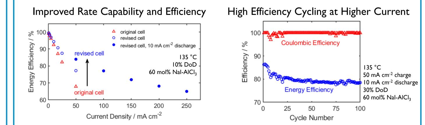
Successfully cycled at 50 mA cm<sup>-2</sup> with charging currents as high as 250 mA cm<sup>-2</sup> possible at 135 °C!
