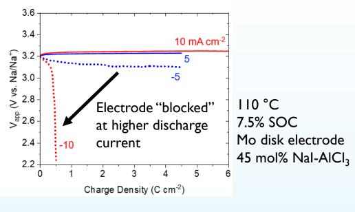
Electrode blocking is reversible and can be avoided at low *electrode* currents. Optimization of electrode area to NaSICON area is needed.
