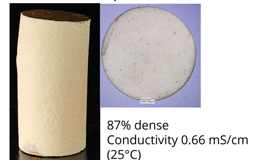
NaSICON ceramic from fully-converted precursor.
