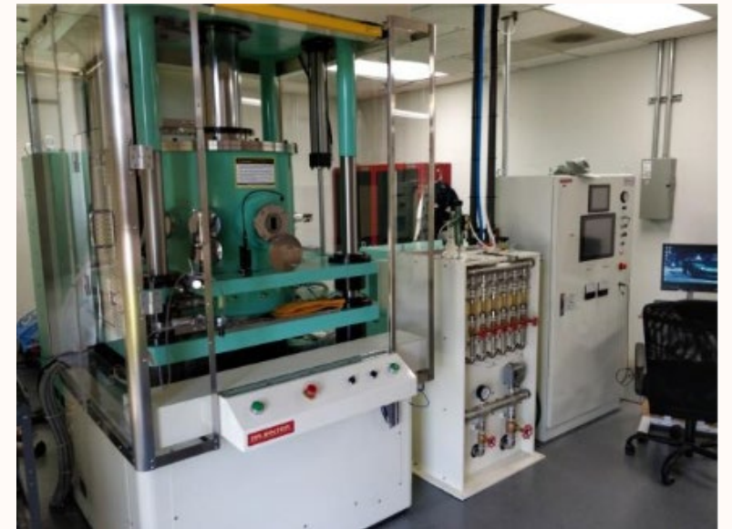
Large scale SPS system at Calnano capable of manufacturing parts up to 6" in diameter
