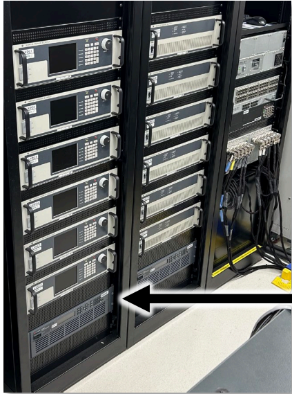
DC Power Supply 500V/40A/10kW
