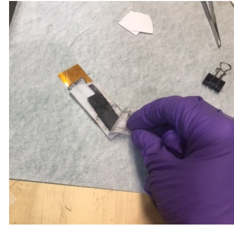
3D Plante cell: Lead foam (ex situ SEM after discharge), combined with an electrochemical half cell (Pb foam, C counter, Ag wire pseudo-reference)
